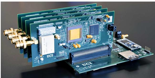
Fig. 8. The core data acquisition system for the 2011 prototype ARIANNA station. Each daughter-card contain an ATWD sampling chip and support circuitry, while the motherboard contains a microcontroller, flash card, and various I/O including USB and trigger inputs and outputs.
