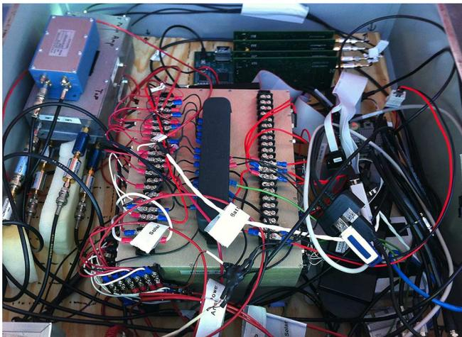
Fig. 10. The 2011 prototype ARIANNA station's data acquisition electronics.
