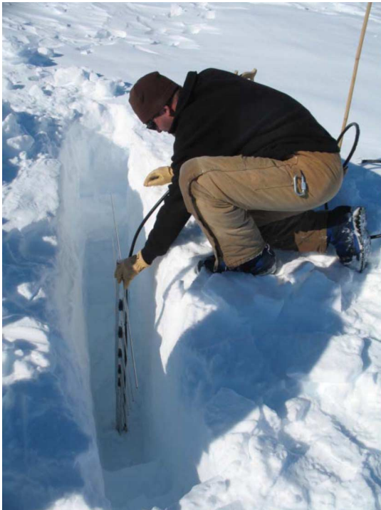
Fig. 4. One of the ARIANNA LPDA antennas being emplaced with the prototype station.
